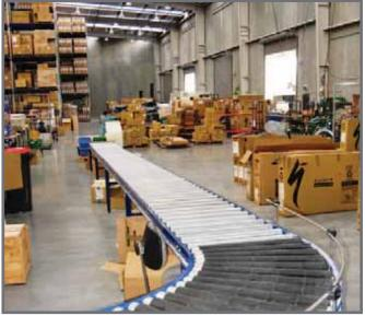
Gravity roller conveyor in bike warehouse
