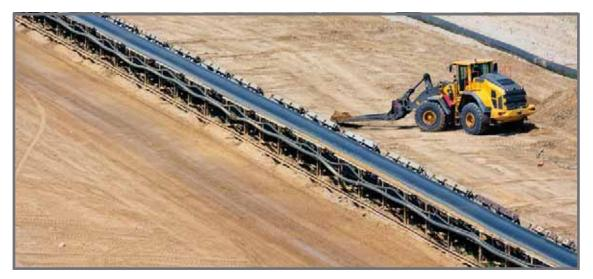
Belt conveyor system in landscape supplies yard - Used for moving soils from one area to another to save tractor travelling
