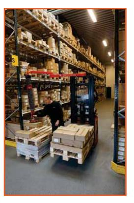
Virtually any load can be lifted using vacuum technology. Suction heads may consist of a single suction cup or multiple suction cups on spreader bar. The positioning may be fixed or variable. Long or wide loads can be lifted using an extended reach control handle.
