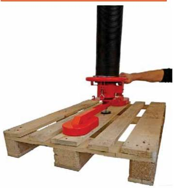
Grabbing and lifting of loads is achieved by the creation of a vacuum within suction heads and a lifting tube. A vacuum pump is connected to the lifting tube via air hose.
