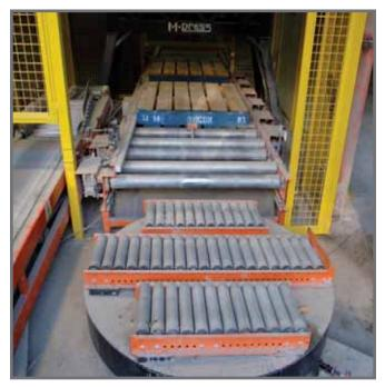
Pallet conveyor for stretch wrapping pallets
