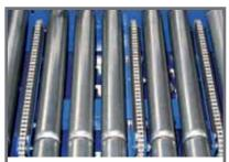
Chain Transfer The chain transfer allows boxes and items to be transferred sideways to another conveyor, packing area etc.
