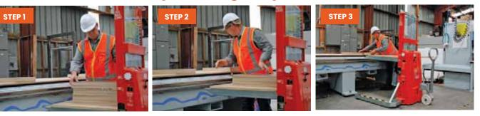
Unloading timber onto conveyor using auto infra-red eye sensor
