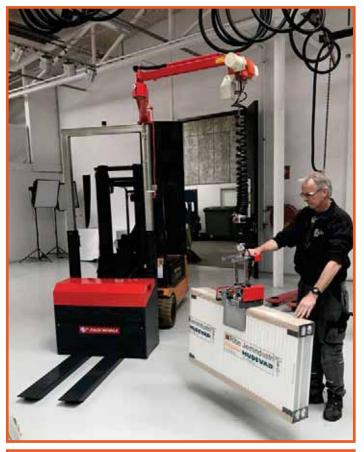
Heavy objects can be moved virtually weightlessly – with only one hand. This virtually eliminates risk of manual handling strain caused by bending, lifting and twisting.
