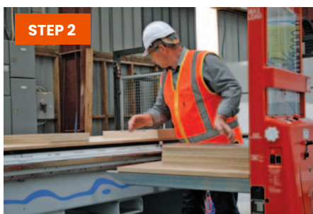
STEP 2 As load decreases the height automatically raises to the conveyor height
