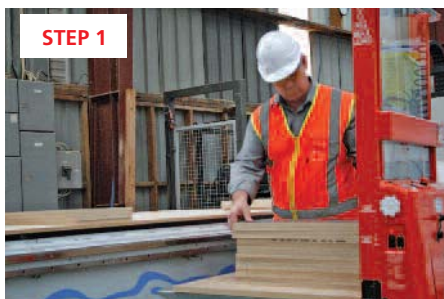
STEP 1 Unloading timber onto conveyor using auto infra-red eye sensor
