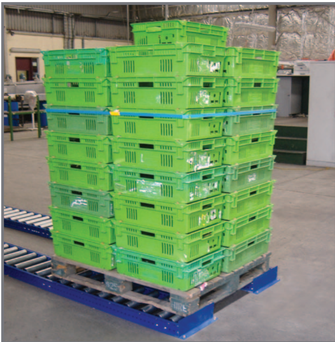
Pallet conveyor mounted to the warehouse floor to transport pallets from the packing line to the pallet wrapping area.
