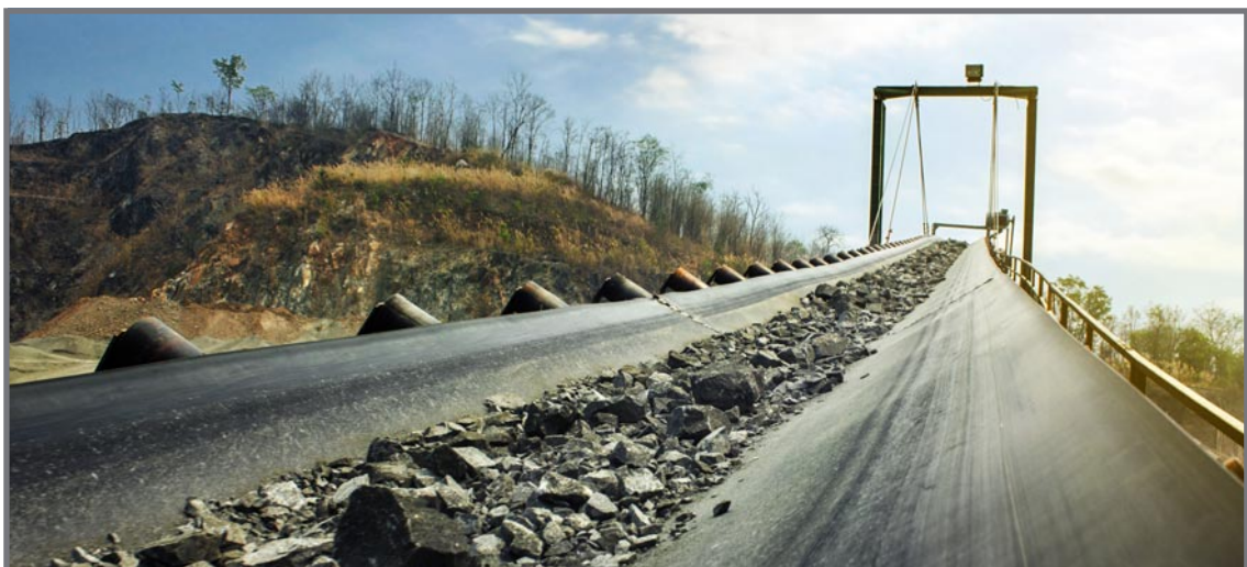
Industrial Belt conveyor system is used for moving coal in mines
