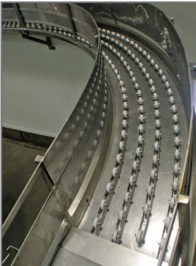
Superfree running skate wheels for empty carton movements
