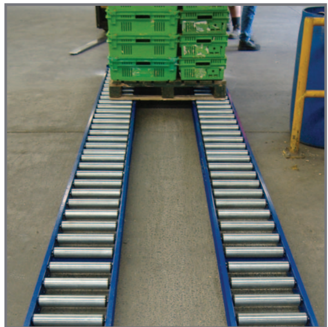
Pallet conveyor mounted to the warehouse floor to transport pallets from the packing line to the pallet wrapping area.
