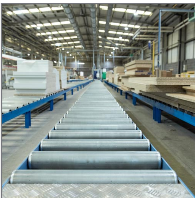
Pallet conveyor for IBC containers to transport to filling station
