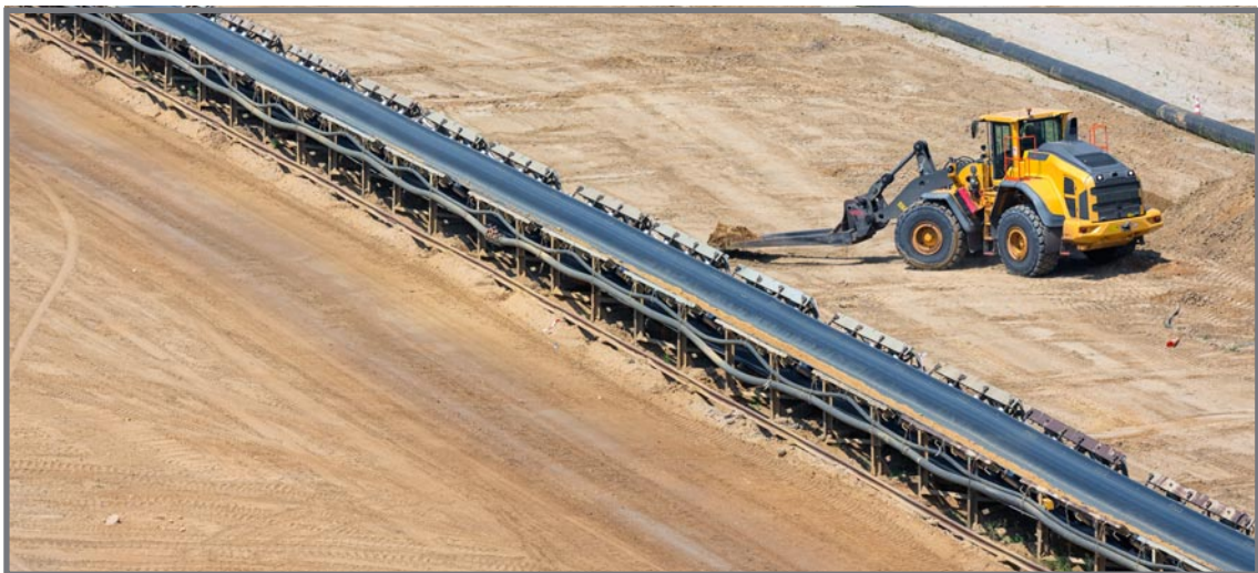
Belt conveyor system in landscape supplies yard - Used for moving soils from one area to another to save tractor travelling
