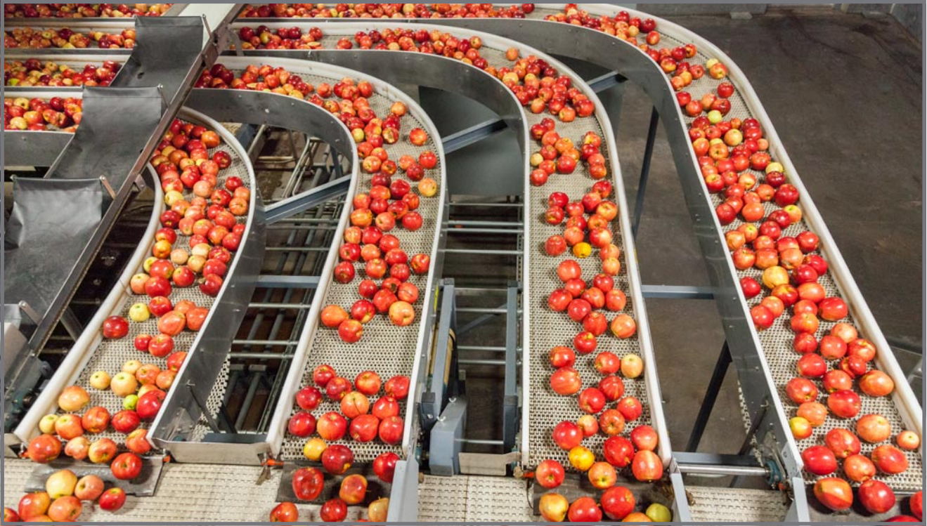
Apple conveyor used for apple sorting
