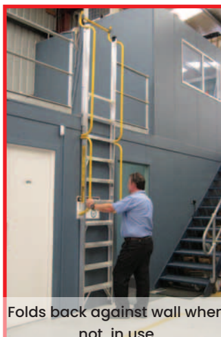
Safety access bar which flips over for access
