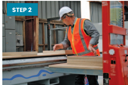
As load decreases the height automatically raises to the conveyor height
