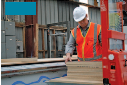
Unloading timber onto conveyor using auto infra-red eye sensor
