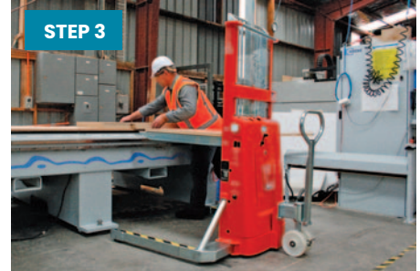
As load decreases the height automatically raises to the conveyor height
