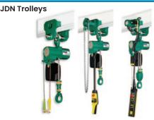
JDN Trolleys are available for both the PROFI and Mining Air Hoists as a manual option (LN) for pushing or pulling by hand. Geared trolleys (LH) are also available for load movement by operating the hand chain mechanism and JDN also offers a motorised trolley (LM) which is powered by an air motor. The carrying capacities go up to 20 tonne.
