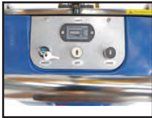
Electric controls to raise and lower unit
