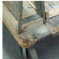
Wood—splinters and rot
