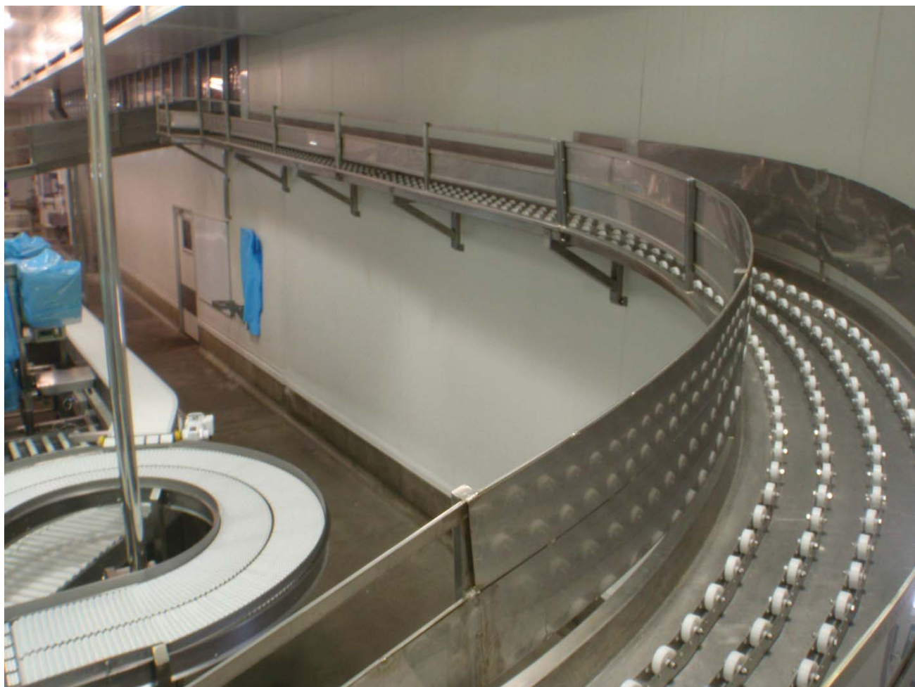
Superfree running skate wheels for empty carton movements
