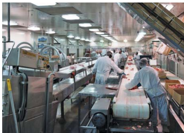
Belt conveyor in meat processing factory
