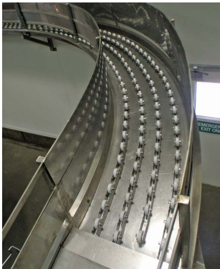
Superfree running skate wheels for empty carton movements
