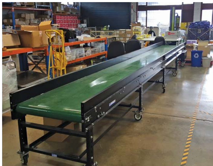
Portable Belt conveyor in warehouse
