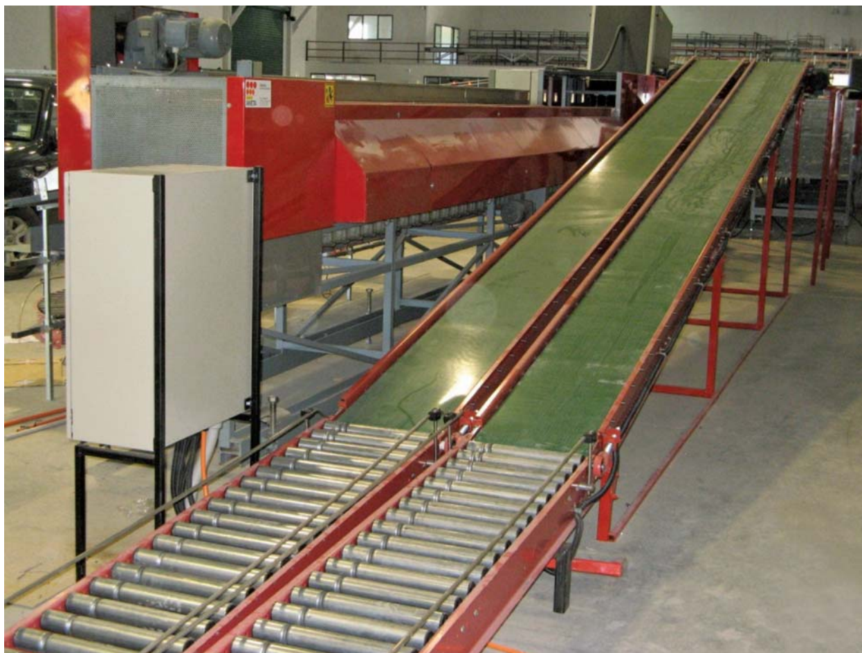
Belt and roller conveyor system in distribution warehouse
