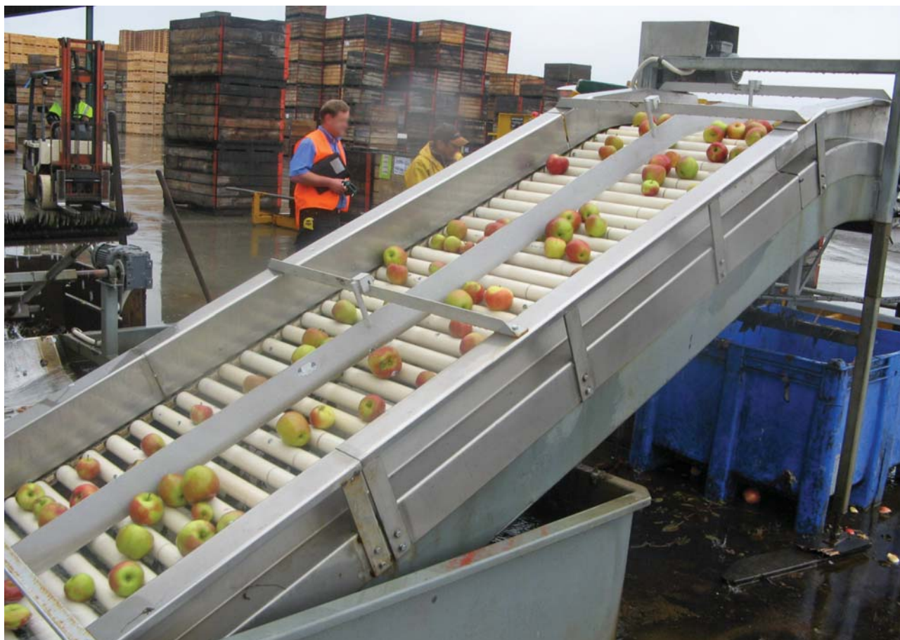
Apple conveyor used for apple sorting
