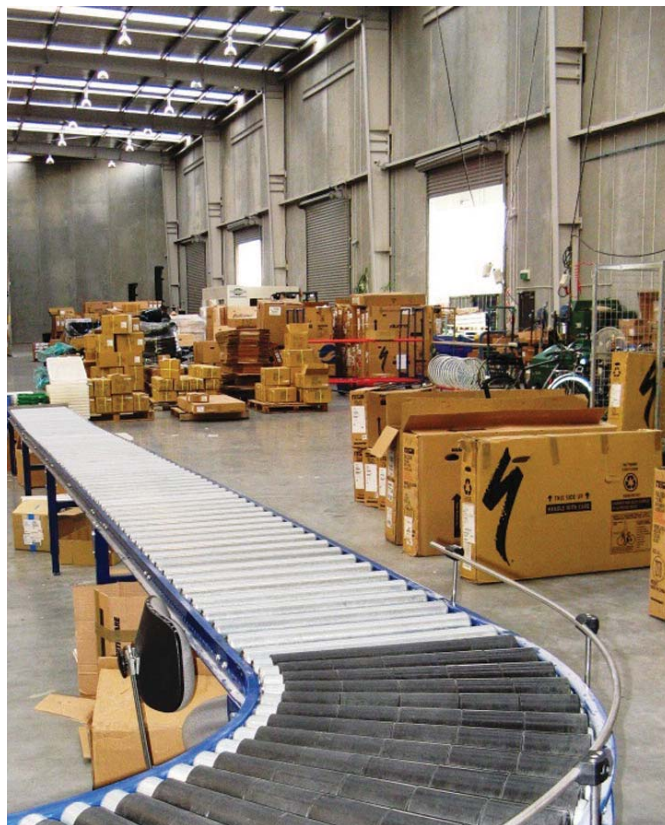
Gravity conveyor in bike distribution warehouse
