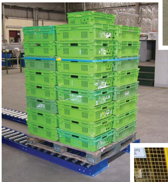
Pallet conveyor mounted to the warehouse floor to transport pallets from the packing line to the pallet wrapping area
