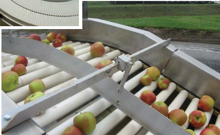
Apple elevator with plastic chain and fully enclosed roller
