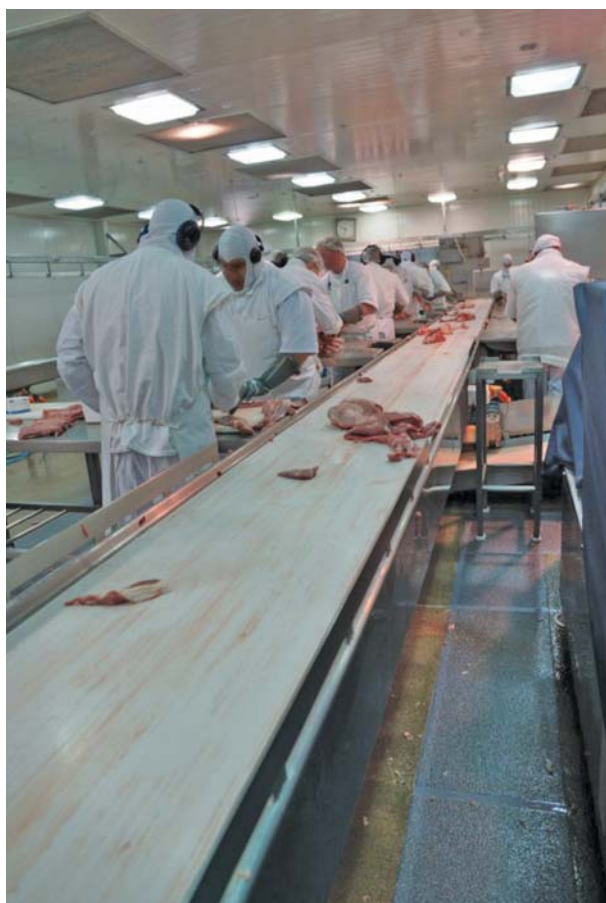
Meat processing belt conveyor system
