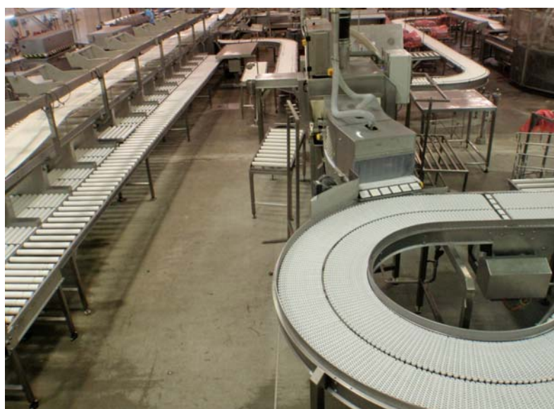
Conveyor system for meat packing room
