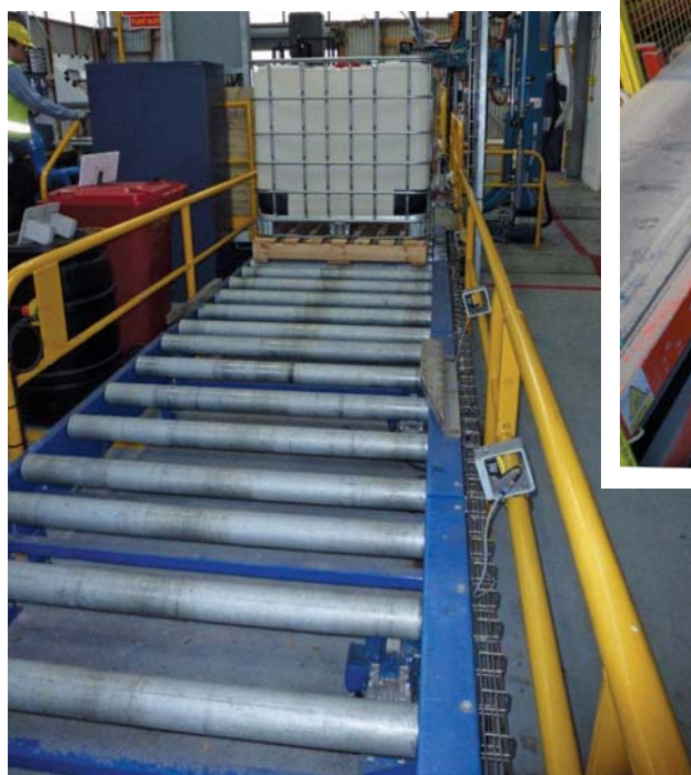
Pallet conveyor for IBC containers to transport to filling station
