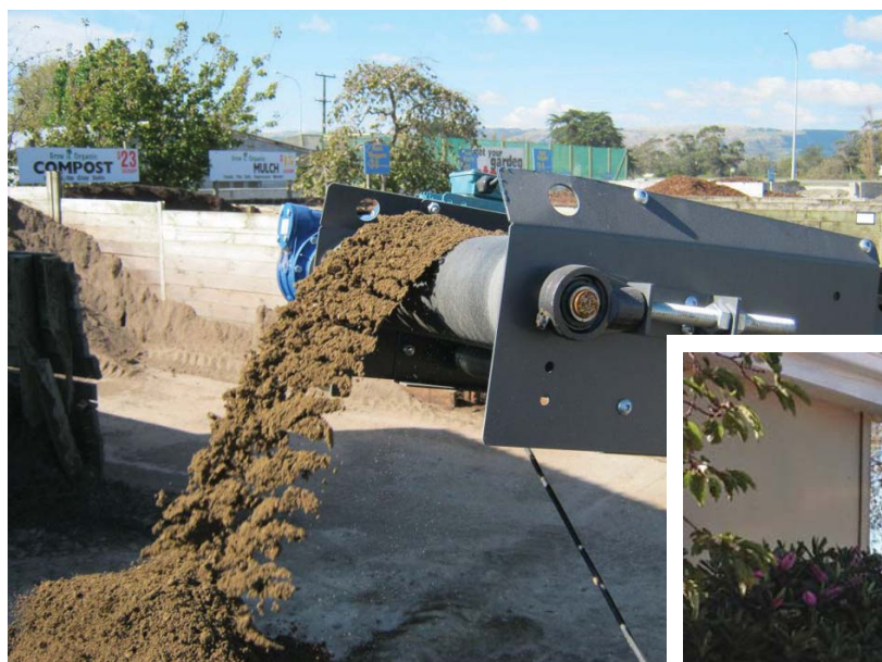
Belt conveyor system in landscape supplies yard - Used for moving soils from 1 area to another to save tractor travelling
