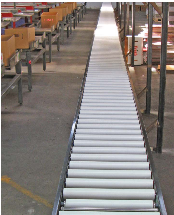
Gravity conveyor apple and fruit sorting warehouse
